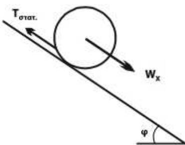
$$\Sigma \vec{\tau}(0) = I_{(0)} \cdot \vec{\alpha}_{\gamma\omega\nu} \Rightarrow T\sigma\tau R = \frac{1}{2} MR^2 |\vec{\alpha}_{\gamma\omega\nu}| \Rightarrow T_{\sigma\tau} = \frac{1}{2} M\alpha_{cm} \quad (3)$$
